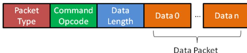
Figure B-2. Packet structure
