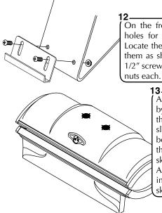
On the front of each leg are two holes for skirt mounting brackets. Locate the two brackets and attach them as shown with two #10-32 x 1/2" screws and two #10-32 locking mute each
