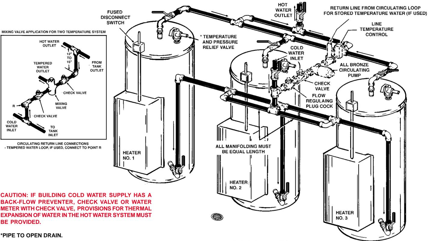
**CAUTION: IF BUILDING COLD WATER SUPPLY HAS A BACK-FLOW PREVENTER, CHECK VALVE OR WATER METER WITH CHECK VALVE, PROVISIONS FOR THERMAL EXPANSION OF WATER IN THE HOT WATER SYSTEM MUST BE PROVIDED.**
