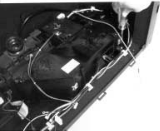
Optical engine screw on right front
