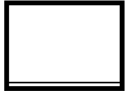
Image too high; adjust both bottom LCD screws together.
