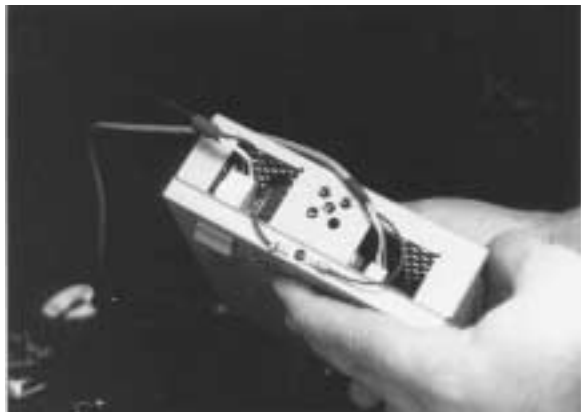
Top of ballast showing two connectors, ground screw, and tabs on the back
