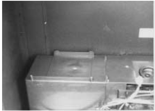
Space where power supply goes, showing tabs at rear and screw sockets in front.
