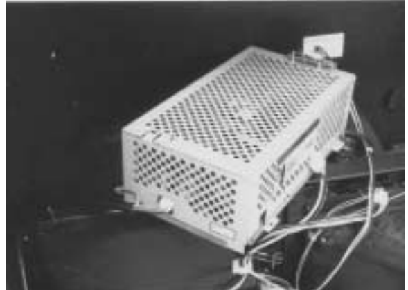
Power supply, partially removed, showing AC input connector on left side; two connectors on right side have been removed.
