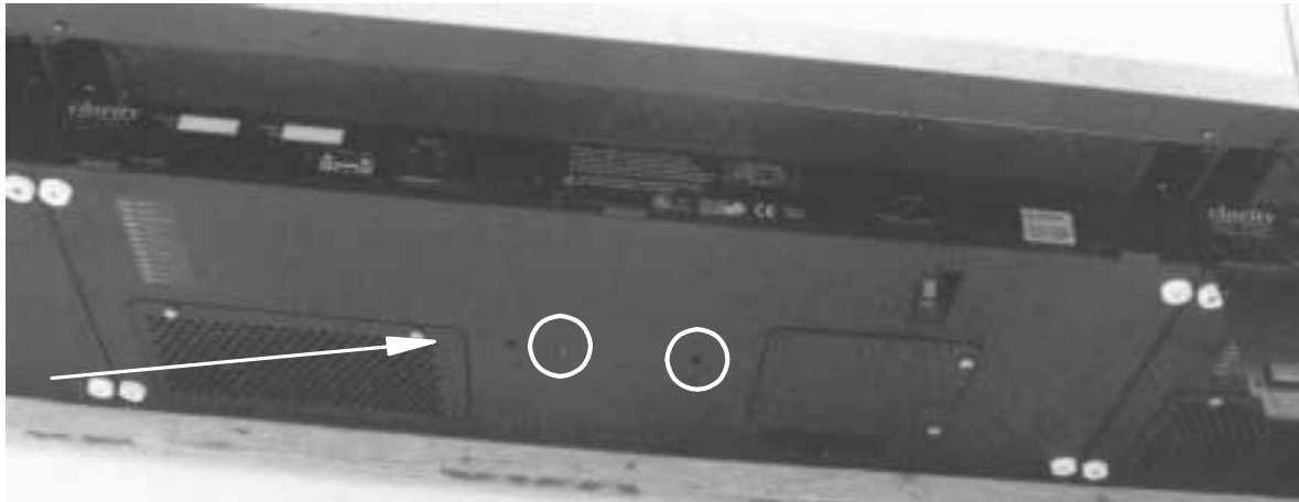
LCD adjustment screw locations: 2 up-down screws in holes shown by circles; left-right screw inside air filter door indicated by arrow.
