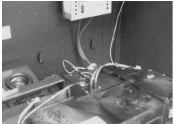
Lamp plug connected and secured with two screws
