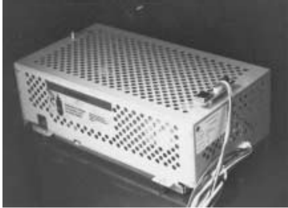
Power supply showing IR sensor on top, two connectors on right; hood has been removed.
