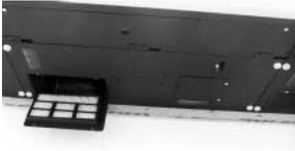
Air filter door opened
