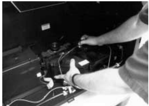
Pull the optical engine forward, then lift it out.
