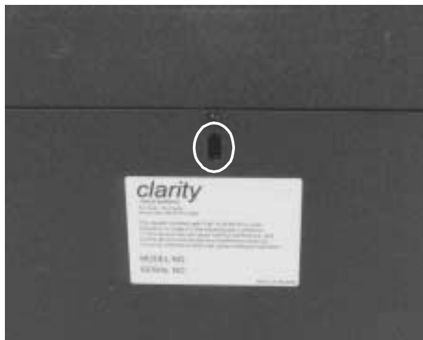
Mirror adjustment screw accessible through hole in rear of display
