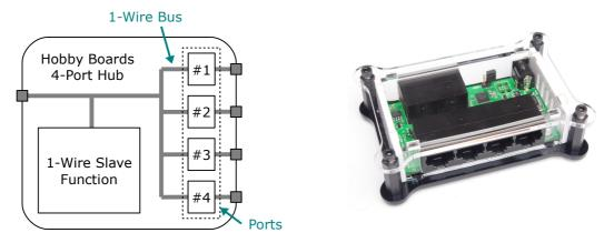
The Hobby Boards 4-Channel Hub adds four sub-branches to a 1-Wire network. The ports are numbered 1 to 4.
