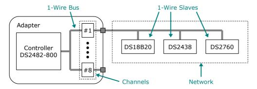
This chapter explains the various concepts in 1-Wire hardware and the way the server works with these concepts.
