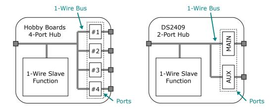
When the server accesses a 1-Wire slave, it makes sure the hub ports that lay on the path from the controller to the target slave are activated first.
