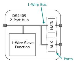
The DS2409 chip adds two sub-branches to a 1-Wire network. The first port is called MAIN, the second one is called AUX.
