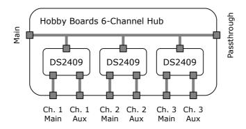
The Hobby Boards 6-Channel Hub incorporates three DS2409 chips. The hub adds six sub-branches to a 1-Wire network.
