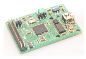
Although the AxiCat technically is a USB to FIFO device, the operating system installs the AxiCat as a USB-to-serial port adapter. As such, label "serial" must occur in client command **Adapter Add** and you've to specify the serial path of your AxiCat.
