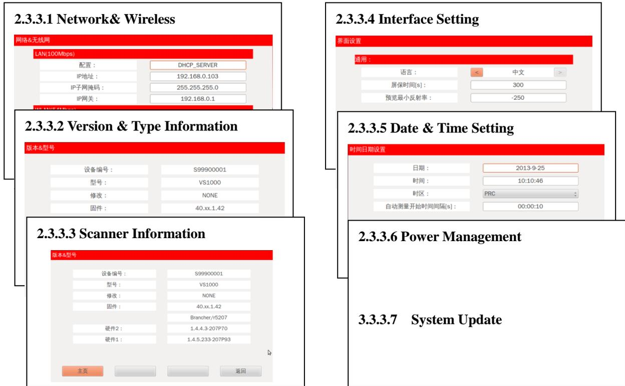
In “System Setting” page the IP address, Language, Screensaver Time, Date&Time can be set, Version, Type and Scanner Information can be looked up, and also include the Power Management and System Update.
