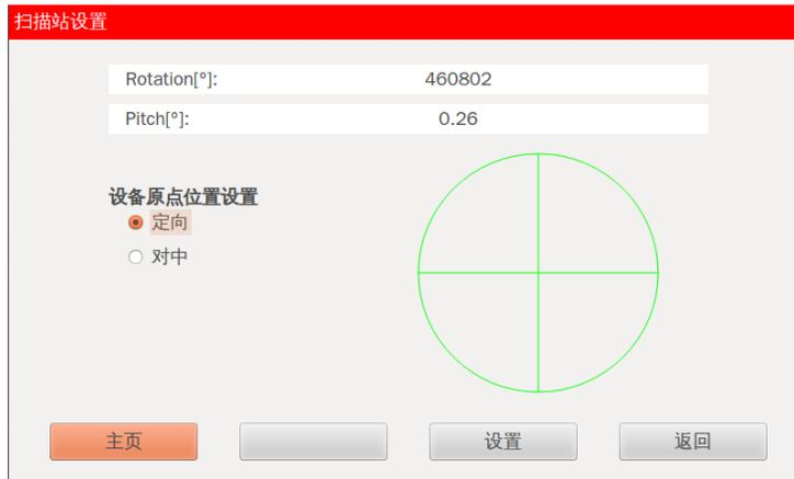
“Position Setting” page for the origin position setting of scanner, choosing “Auto” setting the origin position automatically rely on internal tilt sensor and GPS board or choosing “Input ” manual input the GPS coordinate and tilt data.
