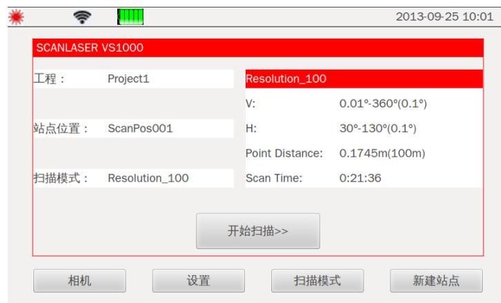
This interface display the settings of the project name, site name, scan mode and other information, “Photo” Button for the camera setting, “Setting” Button for the system setting, “Modes” Button for the corre
