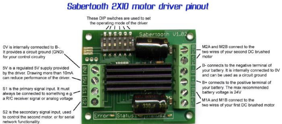
Figure - Sabertooth Pin-out Diagram (Figure printed with permissions by Sparkfun)
