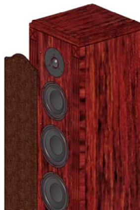
Figure 1: Protective grills are attached to the speakers with a self-centering magnet system. You can remove them by gently pulling them away from the speakers. They can be re-attached by bringing them near to their position on the speaker and the magnets will lock the grills into the right position.
