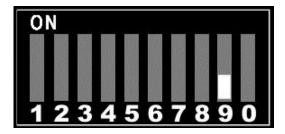
To force audio info to be read from the sink device set DIP switch #9 to ON:
