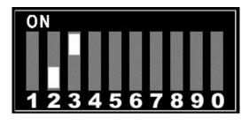
To invert the RGB sync signals, set DIP switch #2 to OFF and DIP switch #3 to OFF:
