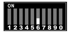
To enable the Power/Status LED, set DIP switch #6 to ON:
