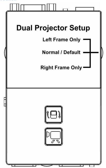
A single HDfury4 set to left or right frame is able to convert 3D content into 2D in case you would like to watch 3D only content in 2D.
