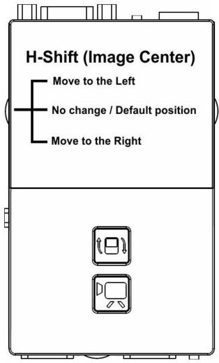
The HDfury4 perfectly centers the image automatically when Component (and/or Digital) video output is used.
