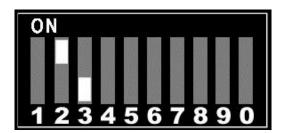
To force the RGB sync signals positive, set DIP switch #2 to ON and DIP switch #3 to ON:
