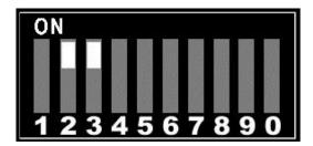
To force the RGB sync signals negative, set DIP switch #2 to OFF and DIP switch #3 to ON:
