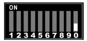
To force video EDID to be set to the built on full 3d HD set DIP switch #0 to ON:
