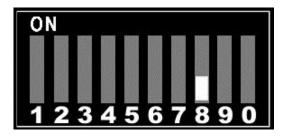
To set 3D output to 720p set DIP switch #8 to ON:
