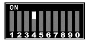
To disable this feature and use normal colour depth (16-235), set DIP switch #4 to OFF:
