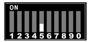
To enable the RGB Shift button, set DIP switch #5 to ON:
