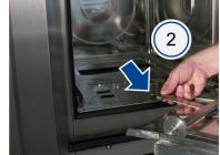
3 Pull the shelf rack onto the transport trolley.
