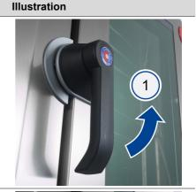
2 Turn the door handle further upwards (2) and open the door slowly.
