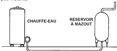
INSTALLATION AVEC CONDUITE D'ALIMENTATION SEULEMENT ET ÉCOULEMENT PAR GRAVITÉ - FIGURE 11
