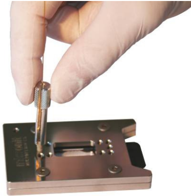
Figure 2.8. Using the extender tool for tightening the fittings
