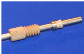
Figure 2.11. Ensure concentricity of compression ring and ferrule
