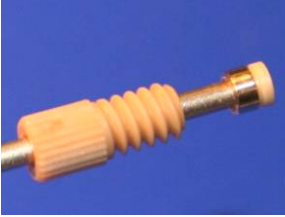
Figure 2.13. Proper assembly of compression ring and ferrule
