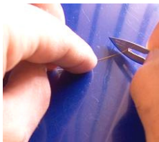
Figure 2.5. Cutting the capillary
