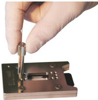
Figure 5.1. Extender tool, for \frac{1}{4} or \frac{1}{3} round additional tightening
