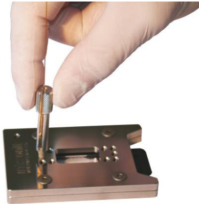
Figure 2.14. Tightening the connection
