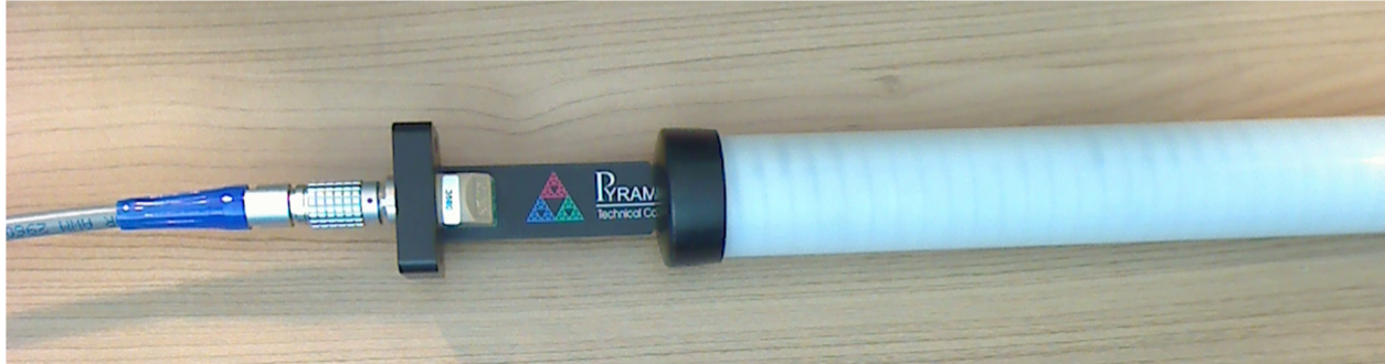
Figure 34. MFP-30 probe in CAL-MFPB0 shield.
