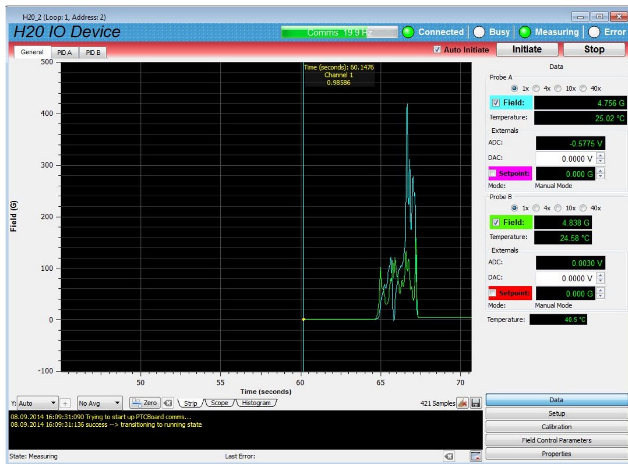
Figure 14. H20 connected and reading magnetic field
