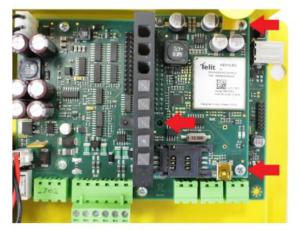
9. Now insert the SIM card and connect the antenna.
