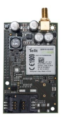
Figure: 2N<sup>®</sup> Lift8 GSM Module
