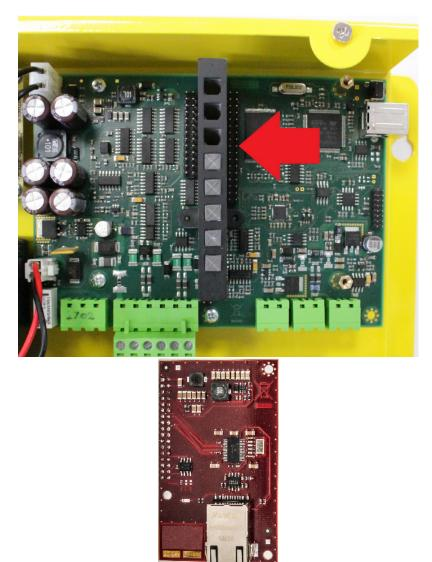
6. Be careful while putting the module on the pins. Make sure that you have connected all the pins to the module connector.
