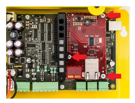
8. Now connect the VoIP line via the RJ-45 connector.
