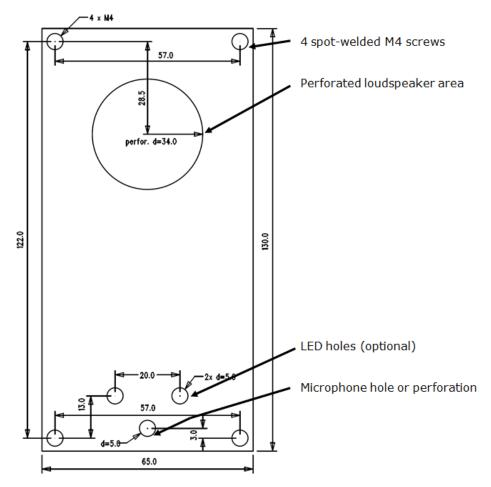
Figure: Mounting Hole Dimensions for Audio Unit – Cabin Universal
