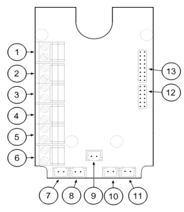
Figure: Terminals, Connectors and Jumpers on Audio Unit - Cabin Universal Board
