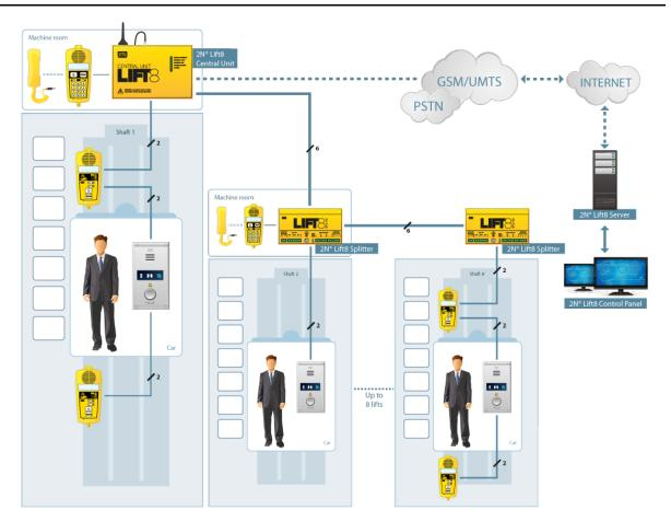
Figure: Example of 2N<sup>®</sup> Lift8 Central Unit, Splitter and audio unit Connection
