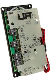
Figure: 2N<sup>®</sup> Lift8 audio unit – Cabin Universal
