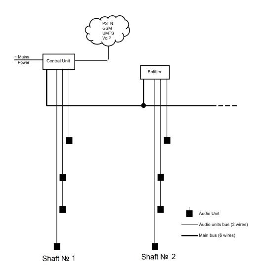
Interconnect the  ${\bf CU}$  and splitter using a 6-wire main bus (power + - , audio + - , data + - ). Mind the polarity.
