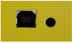
Figure: USB Connector and Reset Button
