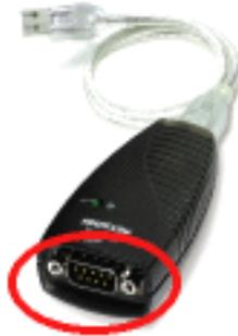
The DB9 port on the Keyspan Adapter is seen as a COM port by Windows. The Keyspan COM port is interfaced via the "Win32 Communications API" and is then available to any program that accesses COM ports via this API.
