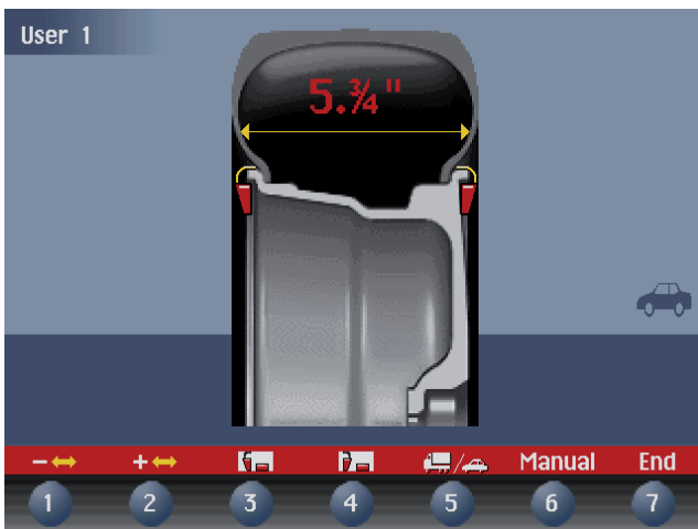
Position of adhesive weights
