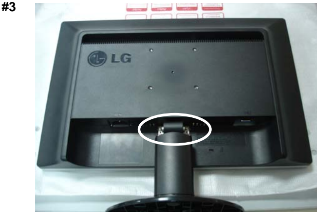
Remove the four screws.
