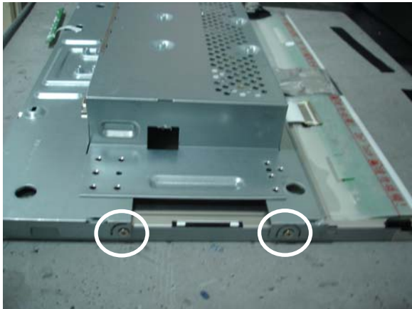
Remove the 2 screws.
