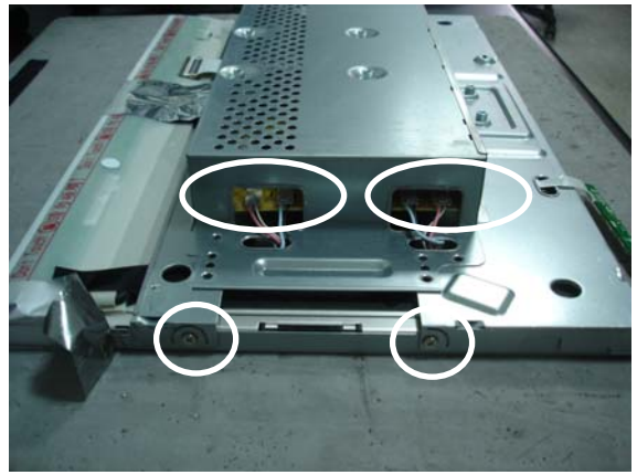
Disassembly the connector and screw.
