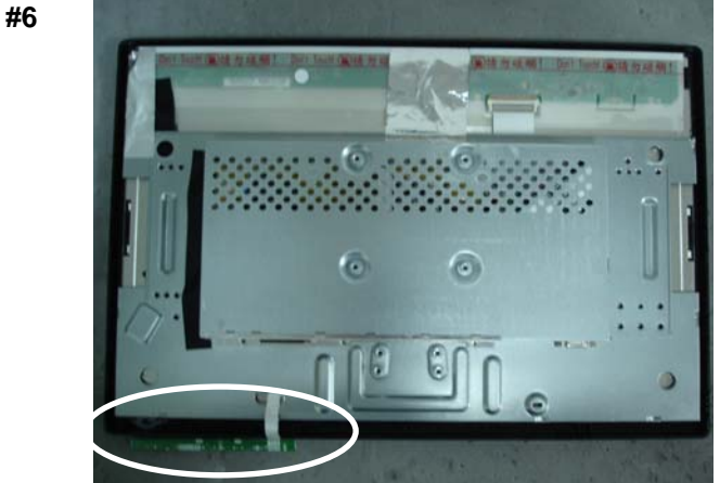
Pull the key board out of bezel.
