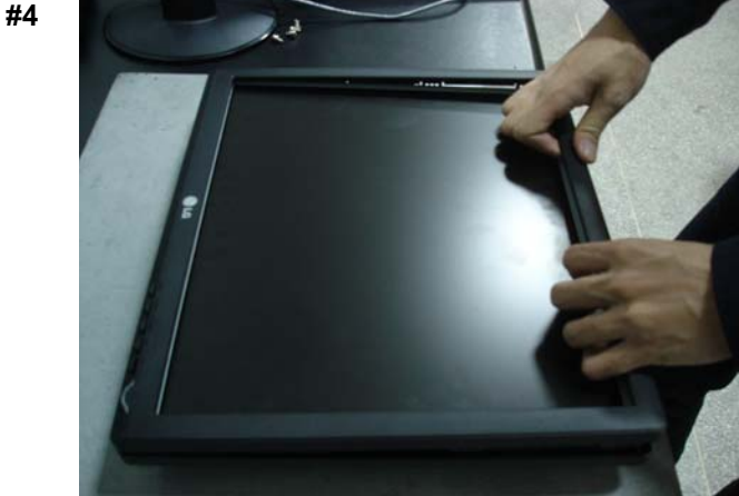
Put the front cover upward. Then let the all latches are separated.
