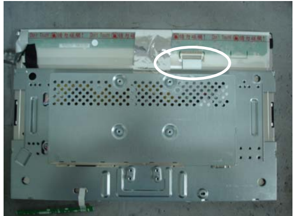
Disassemble the LVDS cable
