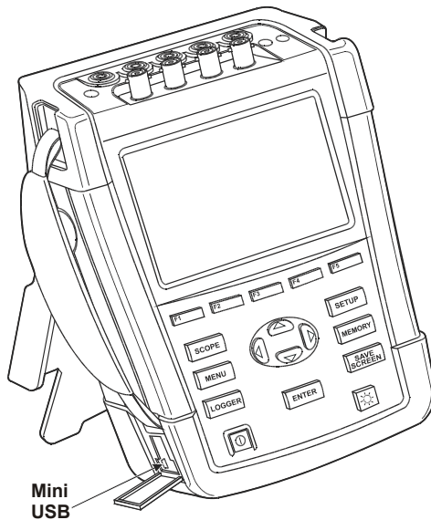
Figure 25-1. Location of USB interface connector
