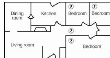
Figure 3: A SMOKE/CO ALARM MUST BE LOCATED BETWEEN THE SLEEPING AREA AND THE REST OF THE DWELLING UNIT AS WELL AS IN EACH BEDROOM.
