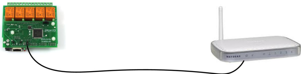
Figure 14. Connecting DAEnetIP4 Five Relay Module to a wireless router.
