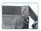
The seat extension post is located inside the seat frame. To access it, insert allen wrench (provided) into screw and turn counter-clockwise to remove screw.
