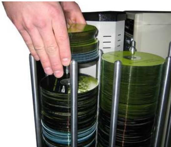
If this doesn't achieve the desired outcome, use an air duster (canned air) to blow air around the circular edge of the blank discs. This process reduces the static between the discs up to 90%. The amount of air to use depends on factors specific to your environment.
