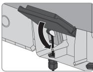
For Sunny Tripower or Sunny Boy / Windy Boy inverters: Tighten the screw of the display assembly.
