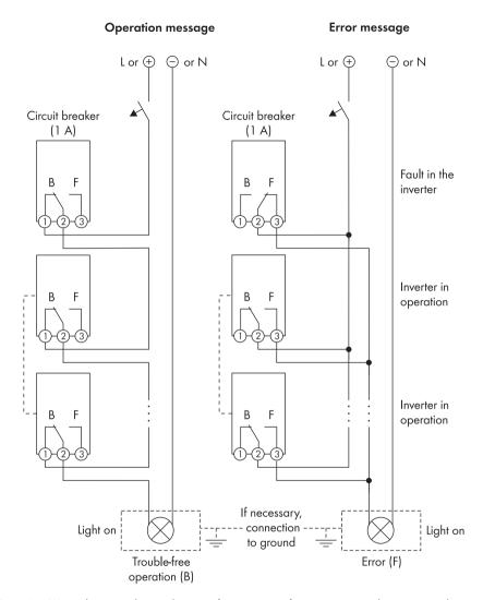
Figure 6: Wiring diagram with several inverters for connection of an operation signaling contact and wiring diagram for connection of a fault indicator contact (example)
