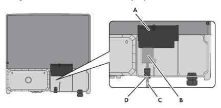
Figure 3: Installation area and cable route in the Sunny Tripower with the lower enclosure lid open and the display assembly flipped up
