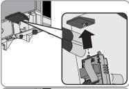
Lead the ribbon cable upwards behind the display assembly.
