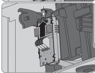
5. Fasten the multifunction relay using the washer and the cylindrical screw (torque: 1.5 Nm). Use an Allen key (AF 3).
