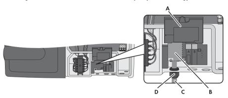
Figure 4: Installation area and cable route in the Sunny Boy Smart Energy with the enclosure lid open and the display flipped up
