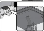
Fasten the multifunction relay using the washer and the cylindrical screw (torque: 1.5 Nm). Use an Allen key (AF 3).
