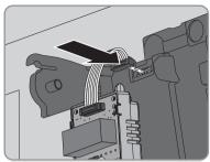
Insert the multifunction relay in the inverter. Lead the left-hand key on the multifunction relay into the hole in the plastic retainer for the display assembly.
