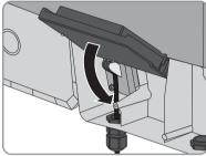
8. Tighten the screw of the display assembly.
