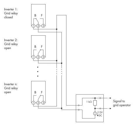
Figure 8: Wiring diagram for reporting the switching status of the grid relay (example)
