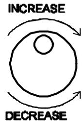
The sensitivity of the control wheel is adjusted dynamically by the EZEAL 5 to suit the type of value actually being changed and the overall sensitivity (speed of response) may be adjusted as desired from the configuration menu (see 5.3).
