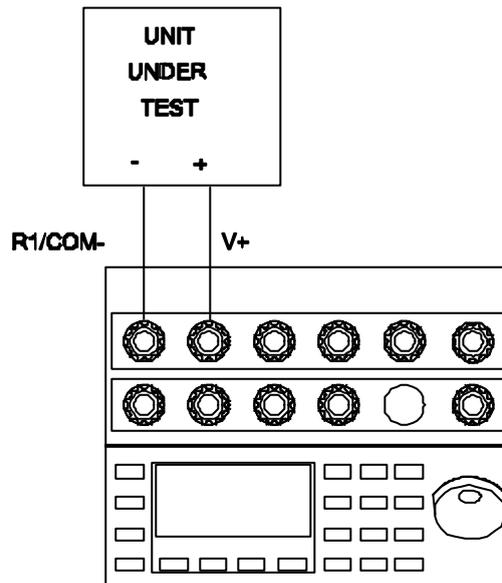
For low level voltage measurements on the 100mV range see section 2.10 for hints on accuracy.
