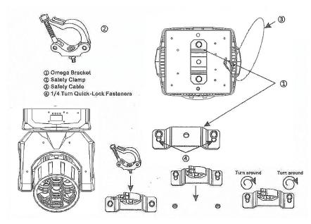
Regardless of the rigging option you choose for your LED super beam, always be sure to secure your fixture with a safety cable. The fixture provides a built-in rigging point for a safety cable on the hanging bracket as illustrated above. Be sure to only use the designated rigging point for the safety cable and never secure a safety cable to a carrying handle.
