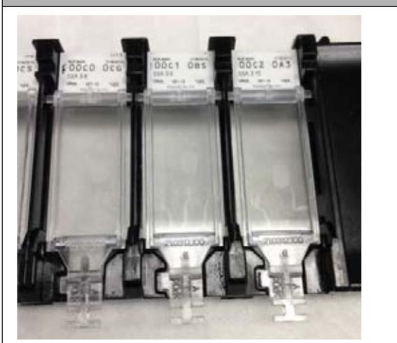
3. Load the slide tray(s) into the processing module and press the Load/Unload button below the tray opening (Figure 5.12).
