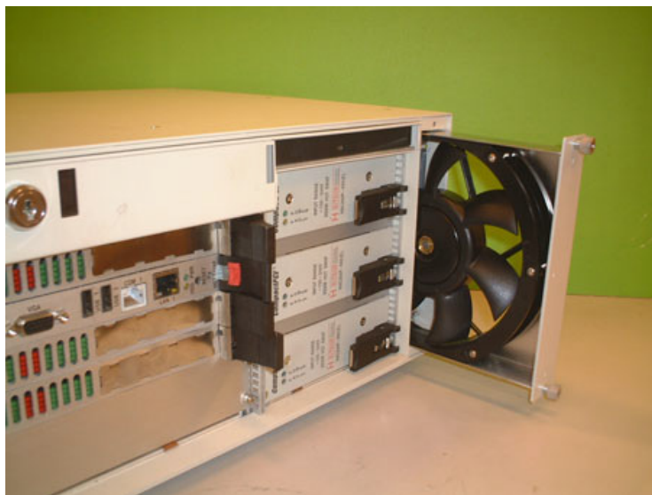
Figure 2.4 Hot-swappable fan maintenance
