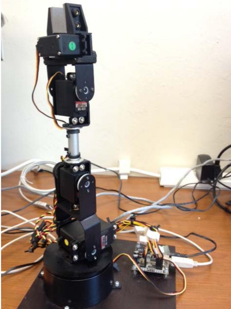
Figure 3 The Lynxmotion AL5A Robotic Arm [4]
