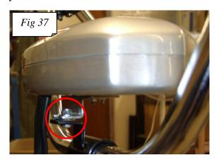
Attach throttle to handle bar: loosened grub screw (2.5mm hex) but do not remove because impossible to re-insert. When throttle is in position tighten grub screw (fig 38). With three small cable ties attach cable to handle bar and under controller (fig 39).
