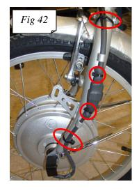
5. Starting from rear, thread main power cable from basket under frame in clips with other cable(s) leaving enough cable to attach plug to battery and secure with cable ties. Excess cable should be at the front to facilitate turning. Cable tie (2 or 3) to make neat (fig 43). Remove all cable tie ends.
