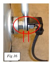
8. Fit anti rotation device to right side front axle with bracket around fork (10mm) (fig 17). Tighten nuts on axle both sides before tightening bracket (18mm). Replace rubber protection cap and fit the black angle bracket onto the axle nut left side. Tighten all front nuts. Check alignment of front wheel.
