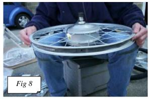
Fit Rear Wheels: for the right rear wheel, locate the 3 pins on axle into the holes on wheel (fig 9). Tighten nuts (22mm). Tap on plastic nut covers (fig 10).
