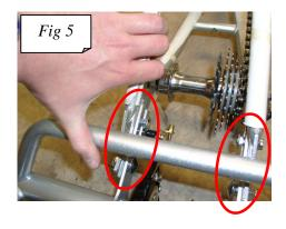
4. Fit small rear chain and adjust it: first of all, ensure cogs are lined up. Then, using chain link tool to insert pin into link from one side until proud (fig 6). After that, swap link over and push pin back a little to allow free movement of link (fig 7). Finally, tighten the chain (do not overtighten: leave around 1cm loose), check alignment and tighten all nuts on rear assembly (14mm).
