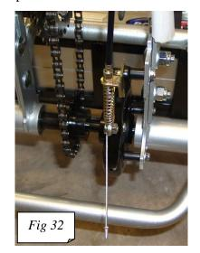
20. Select gear 5 and thread gear cable through frame clips. Attach gear cable to frame with 2 cable ties (fig 33). Secure wire through cable clamp (10mm) and finish cable ends with clamped on aluminium caps (fig 34). Test Gear change movement and ajust it if necessary by turning the adjustment nut located at the end of the cable (at the derailleur side).
