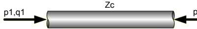
Figure 1: Transmission line components calculate wave propagation through a line using a physically correct separation in time.
