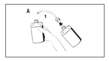
Shake the bottle. Open the fill hose (1) on the bottle (foil seal is thereby punctured).
