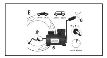
E Open the air hose (5) on the tire valve. Insert the plug (6) into the cigar lighter socket. Then pump the tires (Fig. 7). do not operate the electric air pump longer than 8 minutes! Danger of overheating! If sufficient air pressure is unattainable, drive 10 meters (either forward or in reverse) so that the sealant can be evenly distributed within the tire. Repeat the pumping process. Resume driving immediately, so that the sealant can be evenly distributed within the tire.
