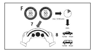
F Adhere the provided sticker to the combination instrument within sight of the driver. Dispose of used tire repair kit at a service station.
