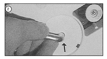
Insert emergency crank (2) as far as possible and hold tightly.
