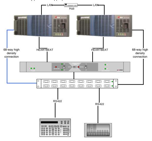
**Important Cloning Note**: To ensure GPI (Input) Configurations do not cause the CLONE playlist to go out of sync, for the Main and Backup device servers, all GPI wiring should be wired to both Main and Clone.
