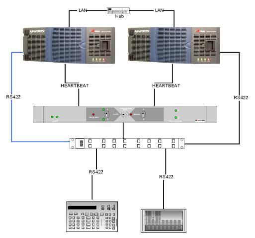
Front panel controls also allow manual change over, as well as providing indication of the current state of the system.
