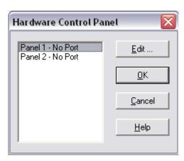
2. Select which COM port the control panel is connect to, and then click on **Edit**. The Hardware Control Panel configuration dialog is displayed.
