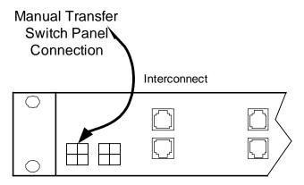
Connection to 8-Port Transfer Switch Relay
