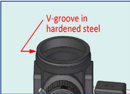
This M55/2" reducer ring is made of hardened tooling steel with an outer V-groove for customized adaption onto a GAM-unit and for archieving shortest possible backfocus with zero flexure.
