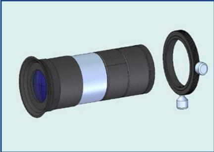
Slide the 1¼" stop ring onto the eyepiece chrome sleeve and lock it.
