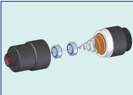
Replace dead batteries with two 1.5V SR41W batteries (#2454306 or #2454307).
