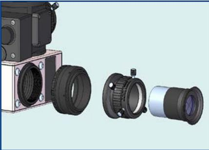
Select the Baader VariLock extension, the 1¼" eyepiece adjustable holder and the 20mm eyepiece.
