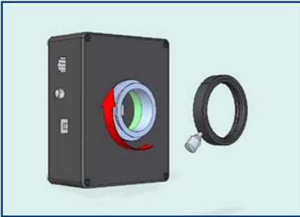
Separate the T-2 Quick Changer and screw the steel part to the detector body. The remaining ring of the T-2 will be attached to the VariLock Extension (see below).
