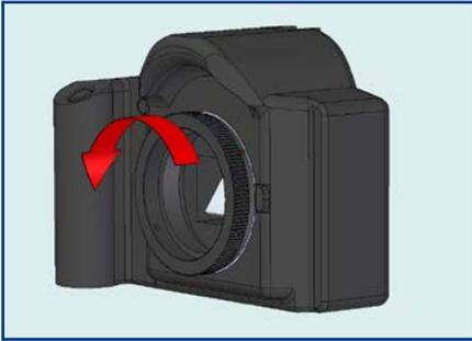
Attach the T ring on the camera body.
