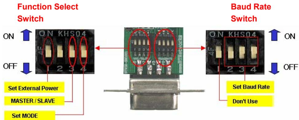
You can select the mode of configuration using pin#4 of the function select switch.
