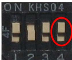
When pin#4 of the function select switch is up, BM1001 will be configured by DIP Switch Only.
