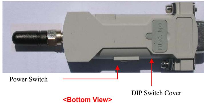
Open the DIP-Switch cover and you may see DIP switch as in below.
