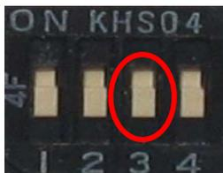
When pin#3 of the function select switch is down, BM1001 is a SLAVE.
