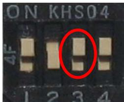
When pin#3 of the function select switch is up, BM1001 is a MASTER.
