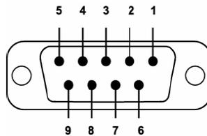
When pin#1 of the function select switch is up, power is supplied via pin#9 of the D-SUB connector.
