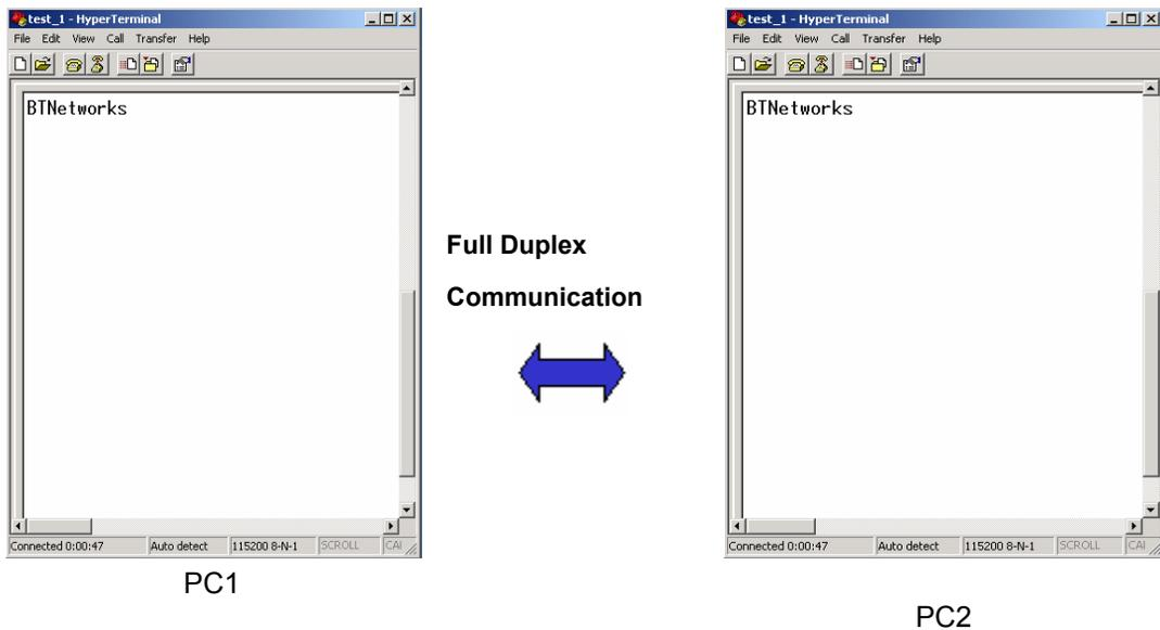
[7] If users may see the characters on both windows, it means data communication both way through BM1001s and setup is successful.
