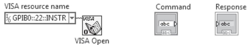
Complete the block diagram as shown next using the VISA icons found in **Functions>>Instrument I/O>>VISA** (and its subpalette **VISA Advanced**). Wire the **Command** control terminal to VISA Write's **write buffer** input and the **Response** indicator terminal to VISA Read's **read buffer** terminal. When executed, **VISA Read** will read up to *N* bytes from the selected resource, where *N* is equal to the integer wired to its **byte count**
