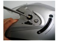
**REMOVAL**: To remove the visor it is necessary to remove the side plates using a screwdriver preferably coated to avoid damaging the paint. Pry between the shell and the plate as shown on the picture, being careful not to damage the paint, then drop the first tooth with the other hand and release the plate. Unscrew the locking screw cap on both sides of the visor, then remove the visor.
