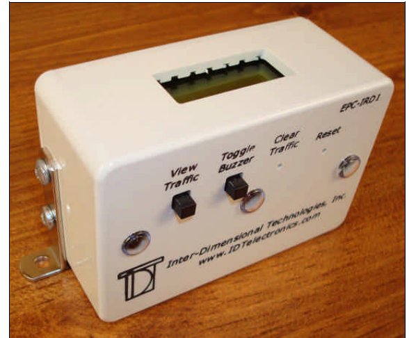
Figure 26b: EPC-IRD1 with "side-firing" brackets installed.
