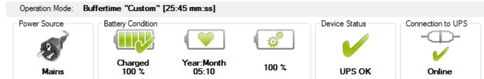
The operation mode in the upper part of the status bar shows the current setting of the buffer time potentiometer of the UPS, as described in topic Buffer time selection (see page 12).
