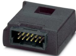
A configuration stick is used to copy parameterization data from/to the UPS device, as described in the topic Configuration stick usage (see page 46).
