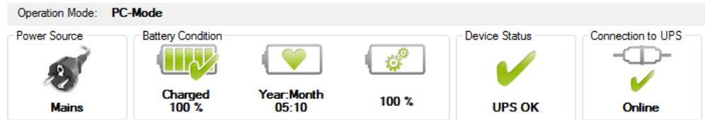
In the "PC Mode" setting on the UPS potentiometer, the UPS functionality follows a chronological sequence that can be parameterized via software, and is thus individually customized to the respective application.
