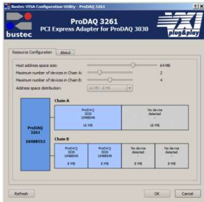
Figure 20 - Adapter Configuration with different Number of Devices and Address Space Size per Chain
