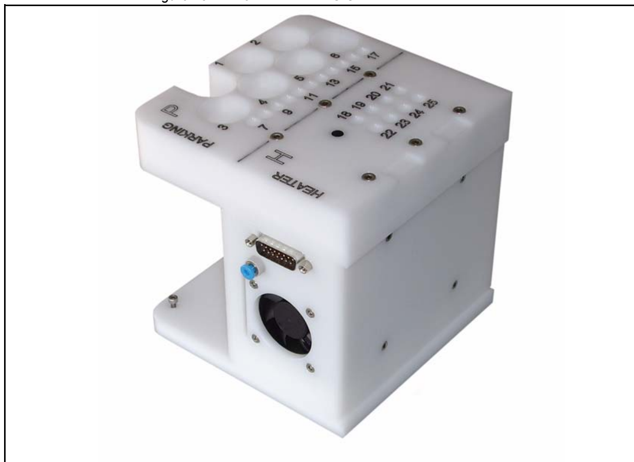
Figure 13.1. The PREHEATING UNIT
