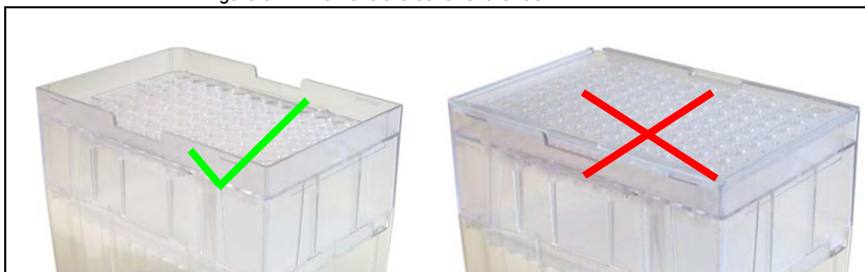
Figure 5.17. Remove the cover of the rack.
