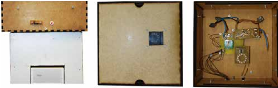
Figure 3.12: The box containing the PCBs of the prototype. Left, the box containing the PCBs, with the UART port and programming button, mounted on the box containing the circuit of the mains. Center, the top of the box with its cover with the windows for the animation. Right, the box without the cover, the PCBs of the prototype are visible.
