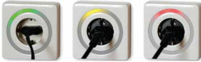
Figure 3.14: The rotating animation of PowerSocket, which change color based on the energy consumption.
