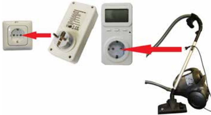
Figure 2.1: The idea of appliance level energy measuring: the energy measuring device is put directly between the appliance and the energy outlet.
