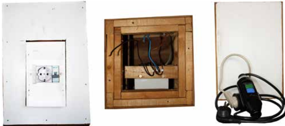
Figure 3.11: The box containing the circuit of the mains of the prototype. Left, the front of the box with the fuse and the socket for the application. Center, the top of the box, the cables which connect to the PCBs of the prototype can be seen. Right, the back of the box, there the plug (white) breaks out of the box. The plug is connected to a ground fault interrupter.
