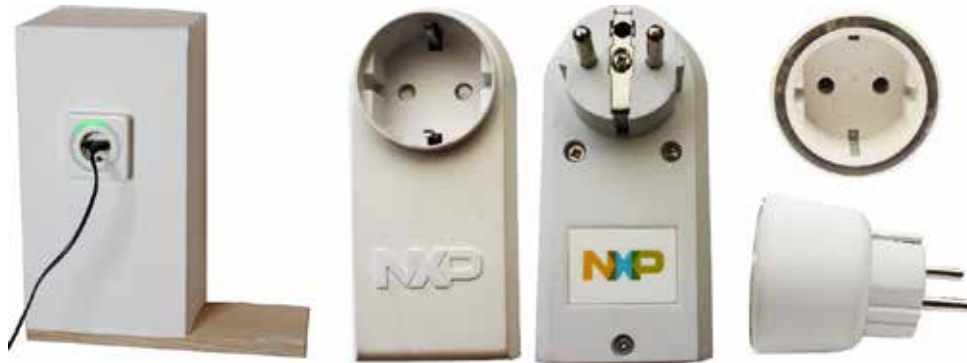
Figure 3.1: The prototypes and products used to construct the prototype. Left, the Powersocket prototype in its present state, a rather large prototype. Center, the EM773 smartmeter from NXP. This device has no power indication. Right, an IKEA night light. It is very small, and has a transparent ring around the socket.
