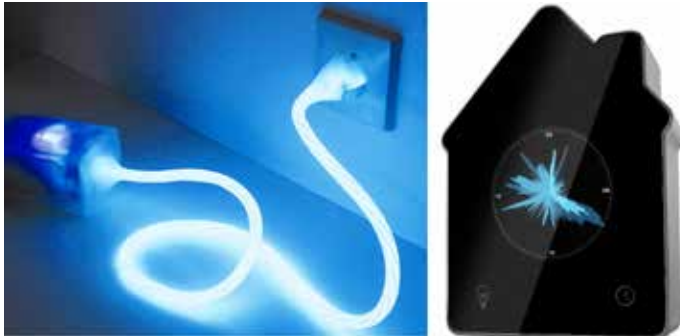
Figure 1.2: Left, the Power-Aware-Cord shows a glowing pattern which indicates a certain energy consumption of an appliance. Right, the Energy-Aware-Clock, is showing a pattern of energy usage. The length of the dial represents the household energy usage at a certain point in time. Both avoid using kWh or Watt as an indicator.
