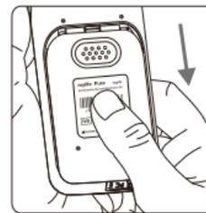
1. Turn the meter over. Press and push battery cover to open.
