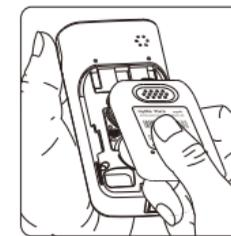
3. Slide the battery cover back until it snaps into place.
