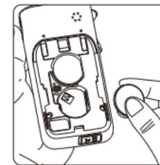
2. Install the battery. Be sure to put battery in correct way with the "+" symbol up.
