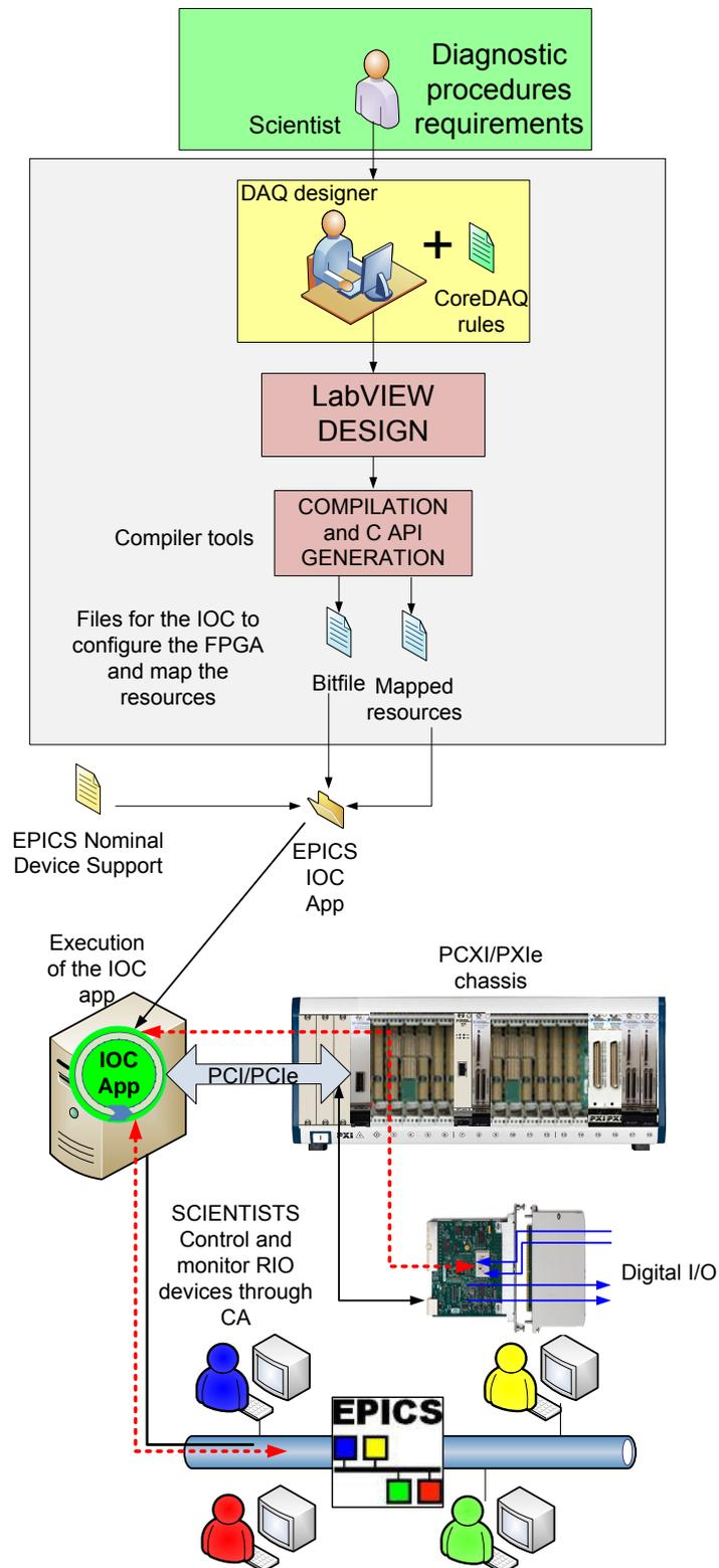
FIGURE 5.1: Main schema of the design cycle workflow. Adapted from Sanz et al. [1]
