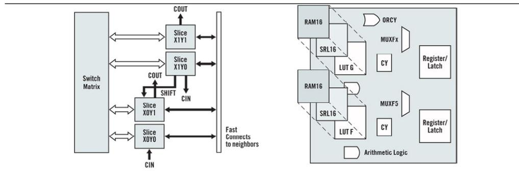
FIGURE 4.2: Configurable Logic Block Structural Scheme [3]
