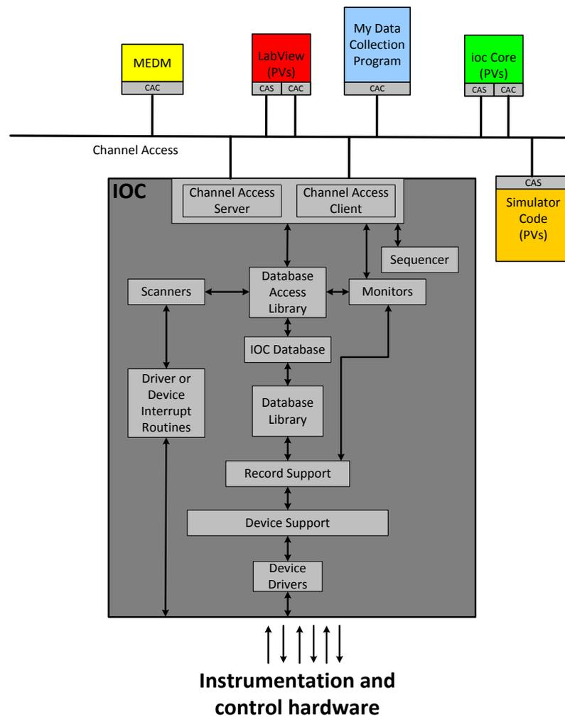
FIGURE 2.2: Generic IOC Exploited View in the Channel Access Network
