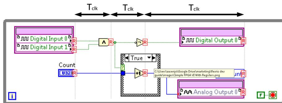
FIGURE 4.4: LabVIEW FPGA While Loop with each function registered,  $T_{clk}$  is the clock period of the system. Extracted from [5]
