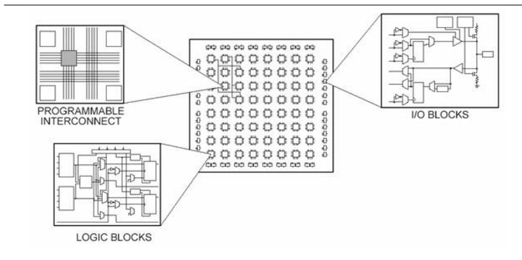
FIGURE 4.1: Scheme of the elements of a FPGA [2]
