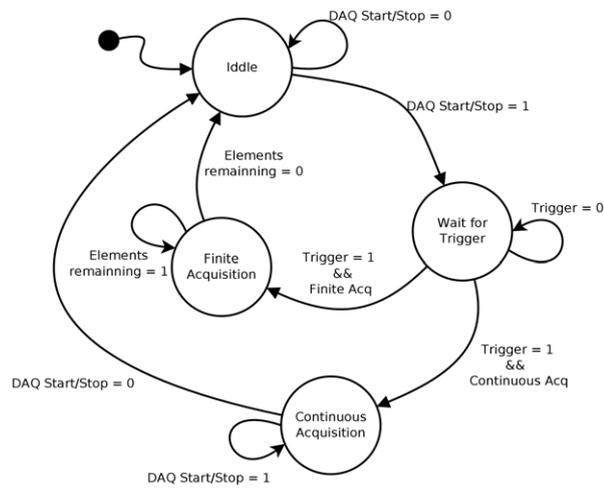
FIGURE 5.9: Automata of the hardware behaviour implemented in the PXIe7965R FPGA
