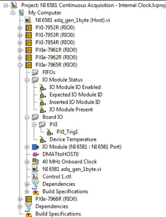
FIGURE 5.8: LabVIEW Multi-target FPGA Project
