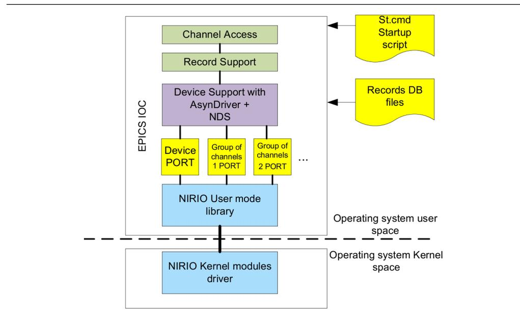
FIGURE 5.11: Software layers of the EPICS driver developed. Yellow coloured boxes correspond to parts of the ndsRIO driver. Figure based on [7].
