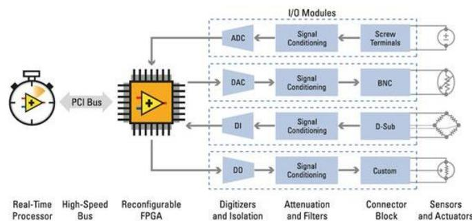
FIGURE 4.3: NI FlexRIO Architecture Diagram [4]
