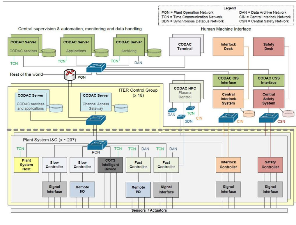
FIGURE 3.1: Physical Architecture of ITER I&amp;C System.
