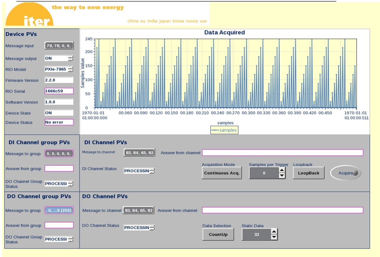
FIGURE 5.13: Operator Interface of the system.
