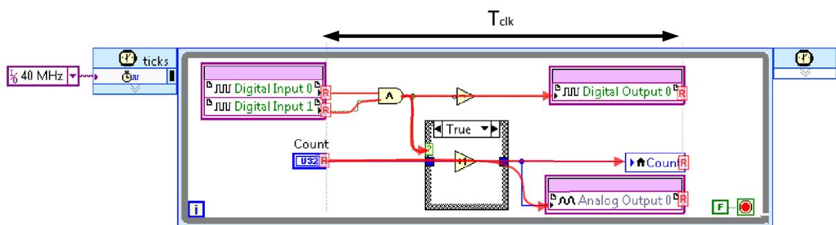
FIGURE 4.5: LabVIEW FPGA Single-Cycle Timed Loop,  $T_{clk}$  is the clock period of the system. Extracted from [5]
