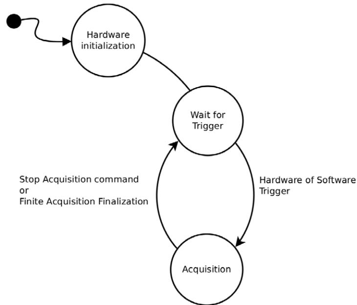
FIGURE 5.12: Data Acquisition Software State Machine.
