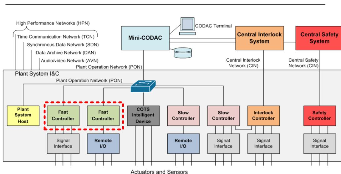
FIGURE 3.2: Fast Controller in the ITER I&C System for PCIe technology.
