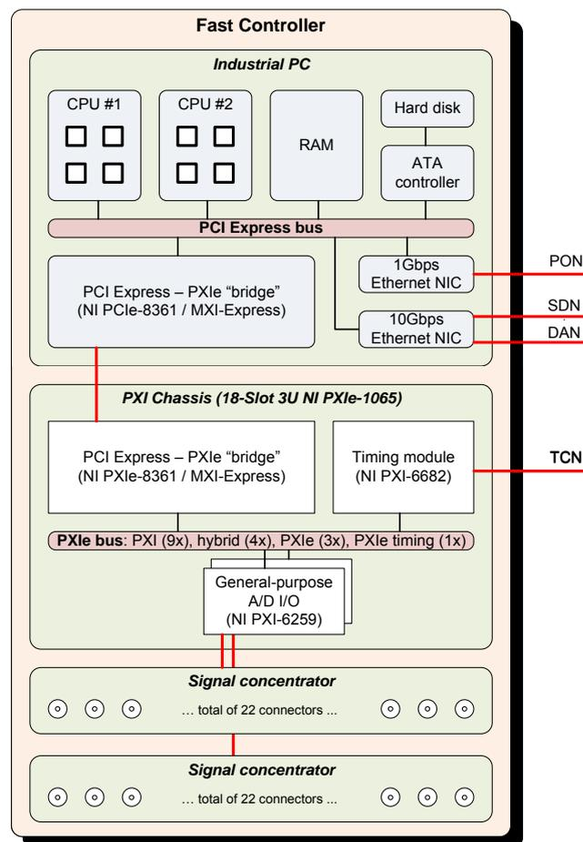
FIGURE 3.3: Fast Controller Physical Architecture Scheme.
