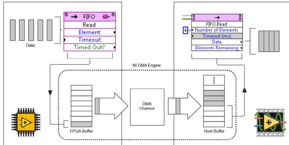
FIGURE 5.5: DMA engine mechanism in RIO technology. Extracted from [5]
