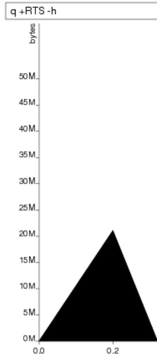
For example, here is a heap profile produced for the program given above in Section 5.1.1:
