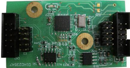
NViS2310 offer an option to integrate the OBDII module, VIOX-CAN01, into NViS2310 system. The form factor of this VIOX-CAN01 is proprietary and it can support either SAE J1939 or SAE J1708 via connection in the first time. The maximum VIOX-CAN01 installed in NViS2310 is up to three units. Please note they are factory option.
