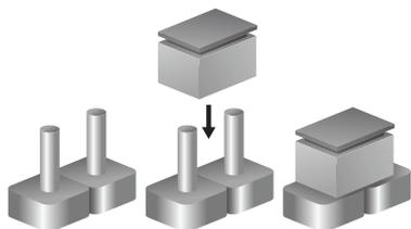
Three-Pin Jumpers: Pins 1 and 2 are Short
