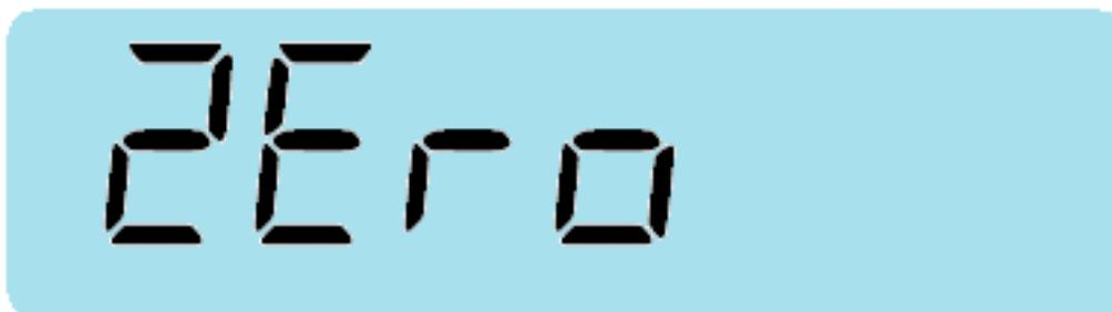
When the pan is empty, press the "Enter" key to calibration the zero value.
