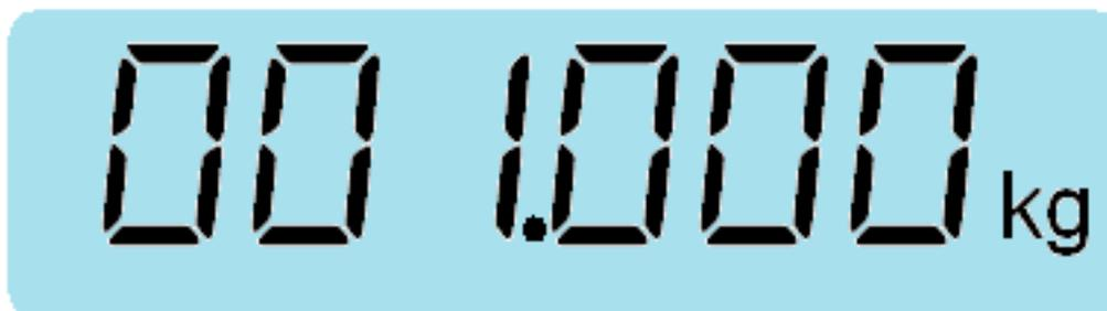
The value of 1 kg has been programmed (using the arrow keys). Put the mass of 1 kg on the pan, let it stabilize, and press "Enter" key. The screen will blink while measuring the weight value.
