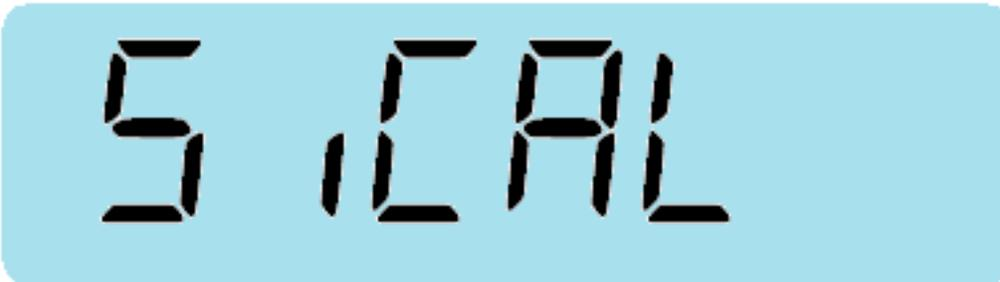
For example, we will calibrate the scale in 3 steps: 0kg, 0.5kg, and 1kg. When the pan is empty press "Enter" key.
