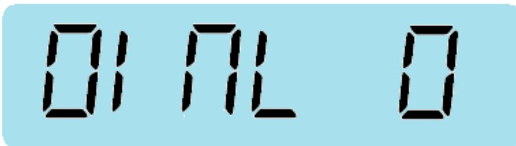
The above mode indicates the scale does not follow the OIML recommendations and the sub-parameters RS, OR and/or OT can be programmed.
