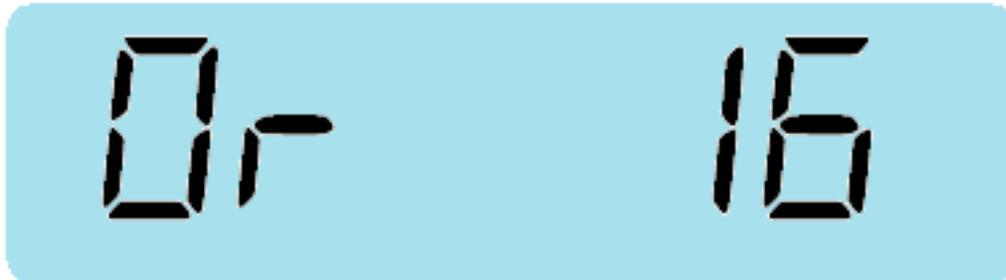
With this configuration of the OR sub-parameter, the scale is capable of starting with an initial deviation of the load cell by 16% from the bottom of the scale.
