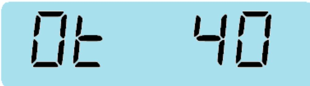
With this configuration of the OT sub-parameter, the scale can absorb the zero drifting which are inferior or equal to 40% of the division value.
