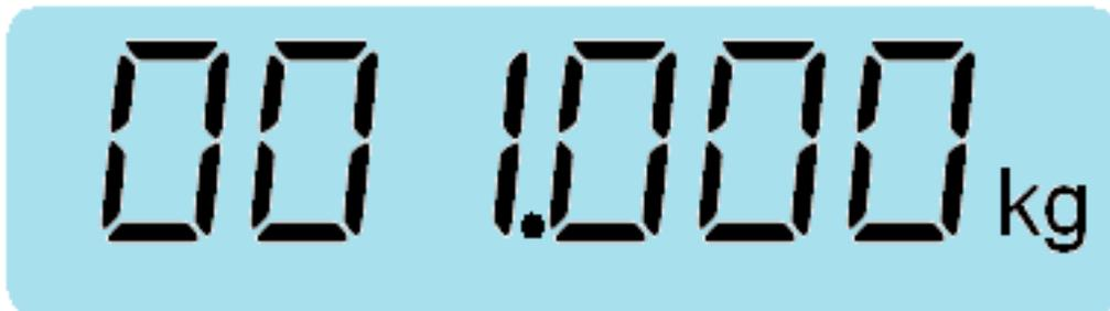
Put the calibration weight (in this case 1kg) on the pan and press "Enter" key.
