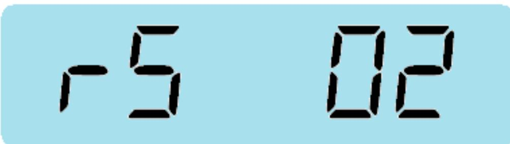
With this configuration of the RS sub-parameter, the scale is capable of absorbing the zero deviation (2% from the bottom of the scale). For example, if the bottom of the scale is 5.000 kg, the scale will absorb up to 0.100 kg by pressing the "Zero" key.
