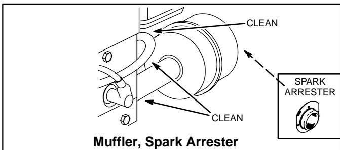
Muffler, Spark Arrester
