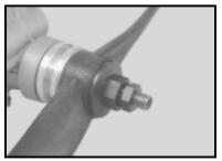
hub to fit the crankshaft. The crankshaft is 1/4" in diameter. Slide the propeller onto the crankshaft and up against the drive washer, then slide the propeller washer up against the propeller. Thread the prop nut onto the crankshaft and tighten it completely to secure the propeller in place. Thread the safety nut into
