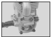
idle stop screw clockwise will make the throttle barrel stay open more. Turning it counter-clockwise will allow the throttle barrel to be closed more. Adjust the idle stop screw so that you can close the throttle barrel completely to shut off the engine. The rotor bolt holds the throttle barrel in the carburetor body and pre-
