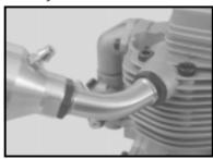
First, thread one nut onto one end of the exhaust pipe, then thread the muffler onto the exhaust pipe. The muffler should be threaded on no less than 1/4" to prevent vibration from damaging the threads. Once you have threaded the muffler onto the exhaust pipe, use an open end wrench and tighten the nut up against the
