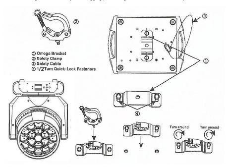
Regardless of the rigging option you choose for the HAWKEYE, always be sure to secure your fixture with a safety cable. The fixture provides a built-in rigging point for a safety cable on the hanging bracket as illustrated above. Be sure to only use the designated rigging point for the safety cable and never secure a safety cable to a carrying handle.
