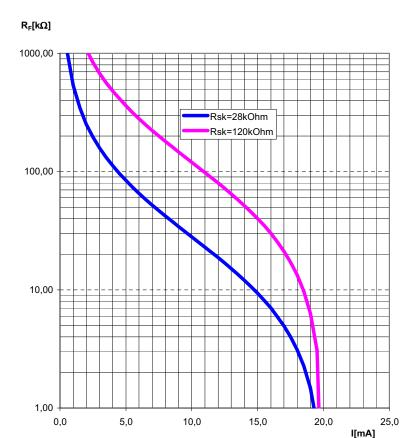
$$R_F = \frac{20 \text{ mA x R}_{Sk}}{I} - R_{Sk}$$
