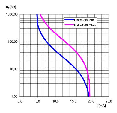
$$R_F = \frac{16 \text{ mA x R}_{Sk}}{1.4 \text{ mA}} - R_{Sk}$$
